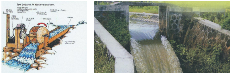
Figure 2.3: Microhydro power system
